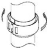
**3** Place the assembled ring on the post and hold in position ready to fit the first MPC clamp which is used to lock the ring together firmly.
