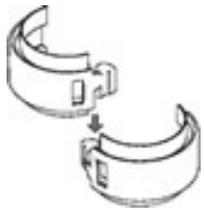
**1** Align the two ring halves one above the other in an open position with the protruding tabs inward, then bring together until each tab sits within the slot on the other.
