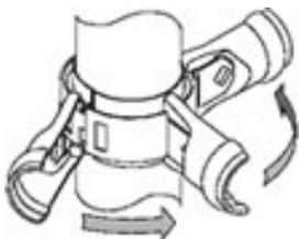
**5** Repeat step 4 above with the second MPC clamp half, this time slide in the opposite direction and again with the open side of the clamp toward the open side of the ring.
